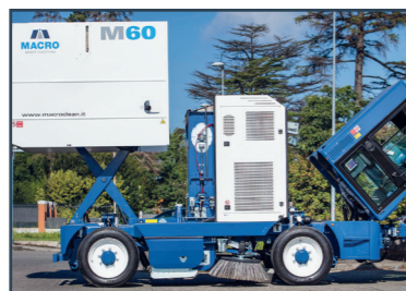
Dumping at any height between 1,1 and 2,3 m.
