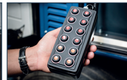
Easy-to-use keypads to operate the machine. "EasyStart" single button for all required functions on/off (CB).
