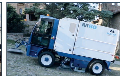
Sweeping and climbing over 20% full-load. The 4-wheel steering gives the M60 excellent manoevrability in all working conditions.
