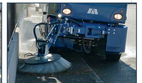
Exclusive capability to sweep in unbalanced conditions (ex. sidewalks). The system allows to sweep on bumps with no operator's action required.
