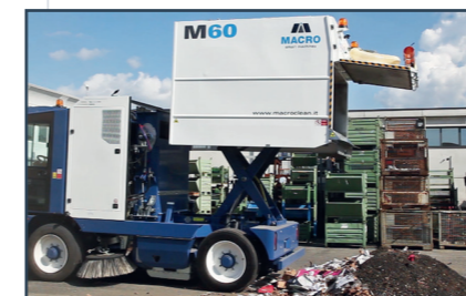
Very large volumes of dry collected waste. 6 m 3 hopper and 6000 kg payload is the highest capacity on the market, allowing long working shifts.
