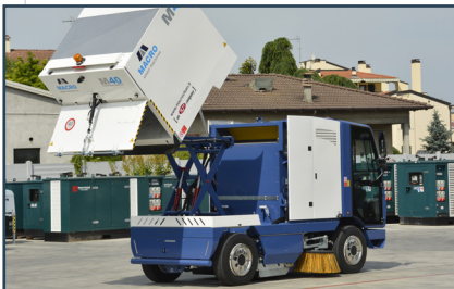
Very large volumes of dry collected waste. 4 m3 hopper and 2600 kg payload is the highest capacity on the market, allowing long working shifts
