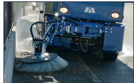
Exclusive capability to sweep in unbalanced conditions (ex. sidewalks). The system allows to sweep on bumps with no operator's action required.
